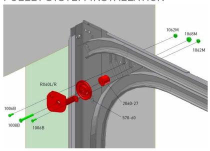
NB! Optional installation of RX80L/R and 570-80 pulley.
