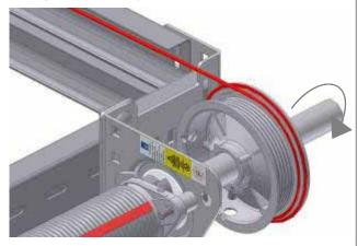
Rotate the drum for winding the cable.
