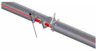
Turn the 1<sup>st</sup> tension lever a quarter turn such that the spring is tensioned.
