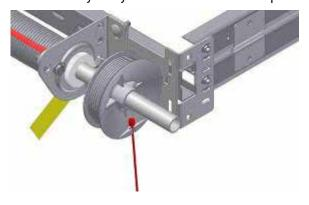
Hook in the cable end in the drum.
