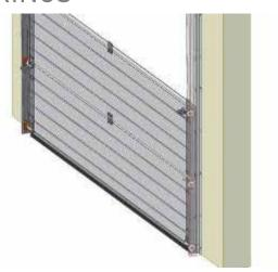
! Cable running behind the rollers to the cable drums
