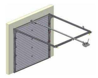
When you have selected an electrical operator drive (LIFTMASTER LM60K/R or other), then this should be assembled in conformity with the handbook supplied with this operator and above displayed instructions. You should clearly follow the instructions for electrical operation in this handbook.
