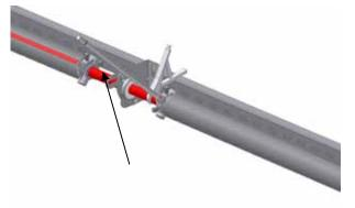
Insert the 2<sup>nd</sup> lever completely into the next slot. Take over the tension of the spring from the 1<sup>st</sup> tension lever to the 2<sup>nd</sup> tension lever. Remove the 1<sup>st</sup> tension lever from the slot. Turn the 1<sup>st</sup> tension lever a quarter turn such the spring is tensioned. Repeat until number of turns is achieved. Then fix the spring plug to the shaft. Check the door balance and adjust the springs if necessary (equally both springs!)
