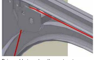
Bring cable trough pulley system to rear.
