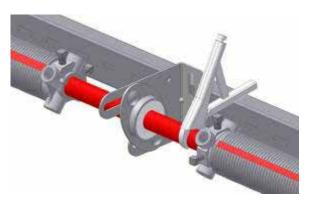
Without key-way: Fix shaft with clamp.
