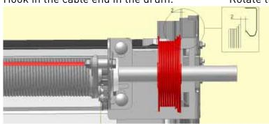
Position the drum on the shaft.
