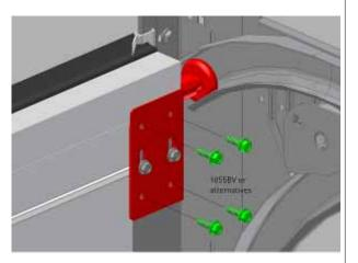
Close the door and secure the door panel. Loosen the two self-tapping screws (1055BV) securing the top roller holder (418SL/R) so that it can be displaced with a slight tick. Press the top panel against the side (upper) seal and slide the top roller holder as far as possible downwards and fix all screws. (minimum play between door panel and seal). The bearing roller lies snugly in the rounding of the bearing tracks.
